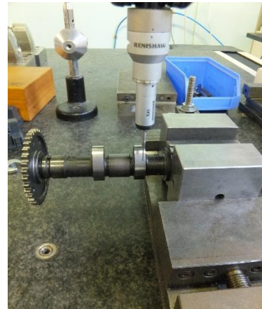
Figure (1): Suzuki SV650 motorcycle engine and its camshaft measurement on a DEA Mistral coordinate measuring machine
